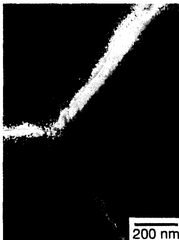
Fig. 4. Example of grain boundary denudation in the CuNiBe with the heat treatment HTC'.
